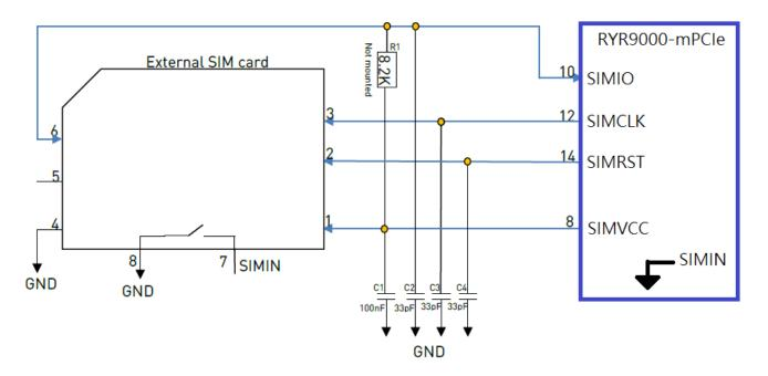
**Note:** The resistor value on SIMIO pulled up to SIMVCC should be defined accordingly in order to be compliant with 3GPP specification. RYW9000\_Series - mPCle contains an internal pull-up resistor on SIMIO. However, the un-mounted option in the application design can be recommended in order to tune R1 if necessary.
