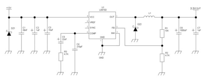
An example of switching regulator with 12V input is in the below schematic:
