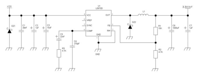
An example of switching regulator with 12V input is in the below schematic:
