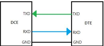
Microcontroller UART @ 3.3V/5V application circuit:
