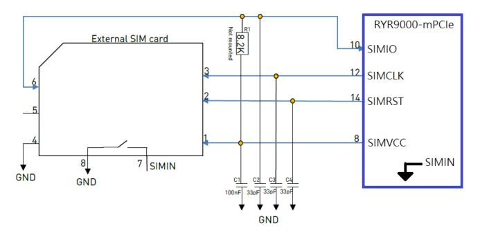
**Note:** The resistor value on SIMIO pulled up to SIMVCC should be defined accordingly in order to be compliant with 3GPP specification. RYR9000\_Series - mPCle contains an internal pull-up resistor on SIMIO. However, the un-mounted option in the application design can be recommended in order to tune R1 if necessary.
